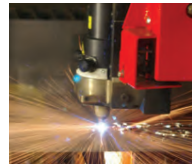
Bystronic Laser able to cut up to 25mm thick mild steel
