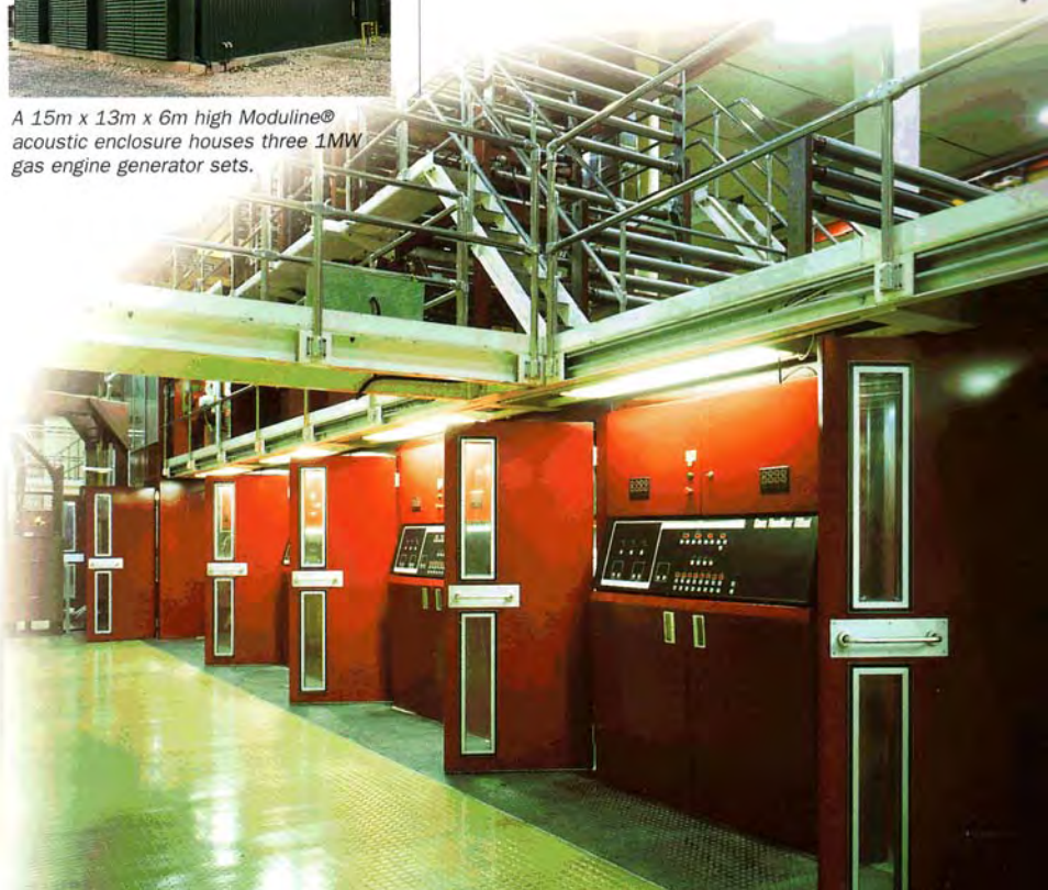
Close-fitting Moduline® barriers control noise emissions from newspaper printing presses.
